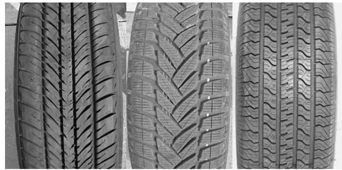
Figure 4. Photograph of the Aquatred (left), Dunlop (middle), and SRTT (right) test tires.
