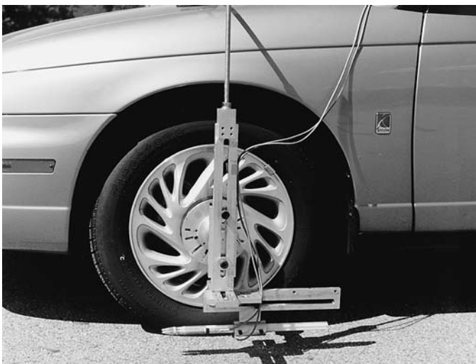
Figure 2. OBSI single probe position opposite the leading edge of the tire contact patch.
