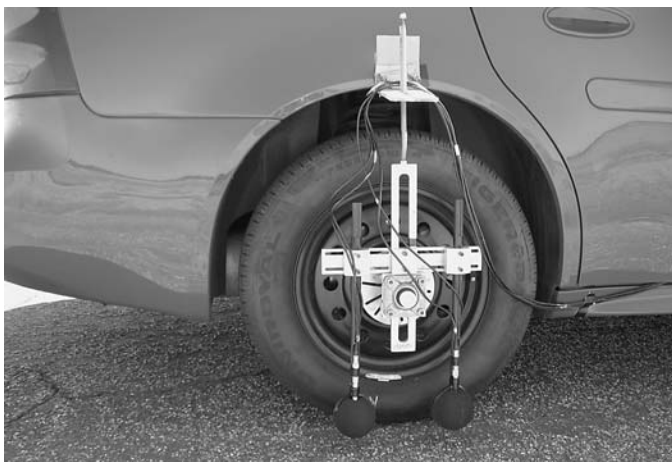
Figure 8. OBSI equipment installed on DPG test vehicle.
