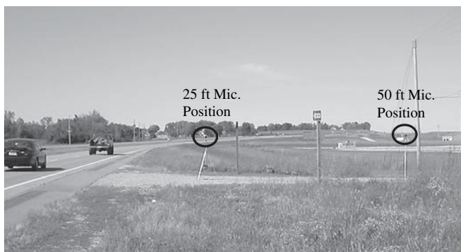
Figure 12. Typical passby measurement setup.
